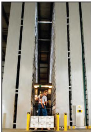
Stoffel Equipment Company, the Raymond Dealership in Milwaukee, WI and Spacesaver Corporation of Fort Atkinson, WI have integrated Raymond's Very Narrow Aisle (VNA) equipment with Spacesaver's newest rack design, the XTend™ Mobile High Bay Storage System (patent pending).
